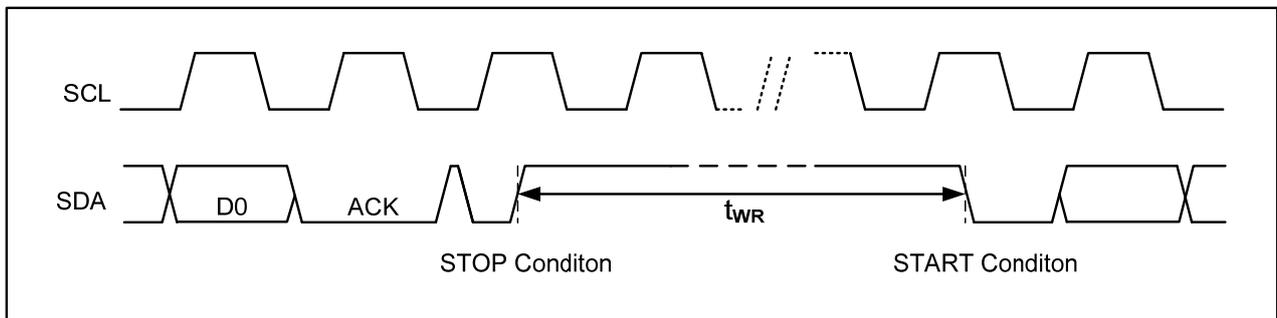
Note: The write cycle time  $t_{WR}$  is the time from a valid stop condition of a write sequence to the end of the internal clear/write cycle.
